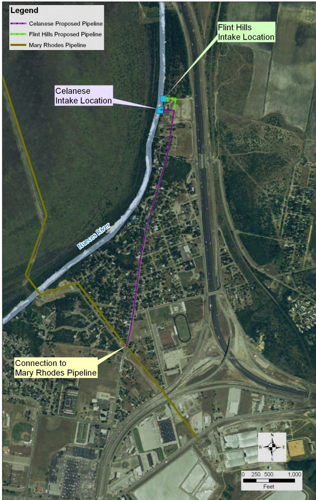
Figure 5D.3.42. MRP Interconnect Pipeline Route
